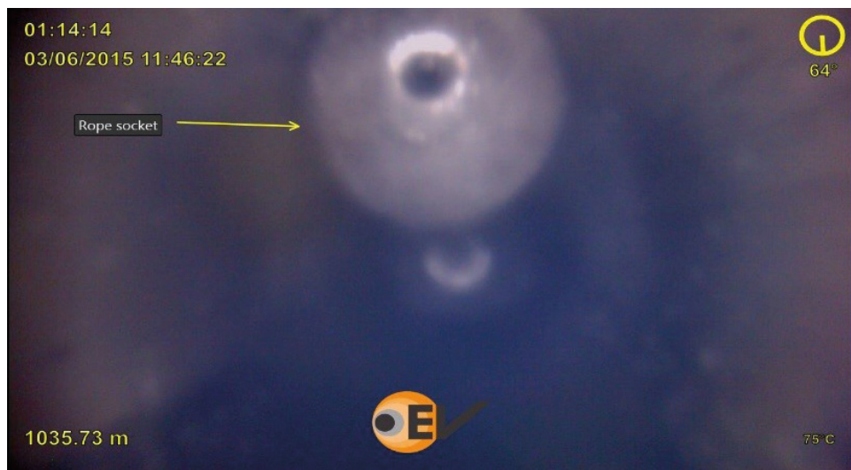
Figure 1: Drop bar fishing neck sitting on the low side of the wellbore and located at 1035 m
