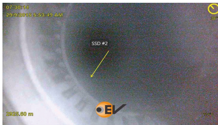
Figure 4: Confirmation of SSD#2 open position during a coil tubing intervention in treated sea water
