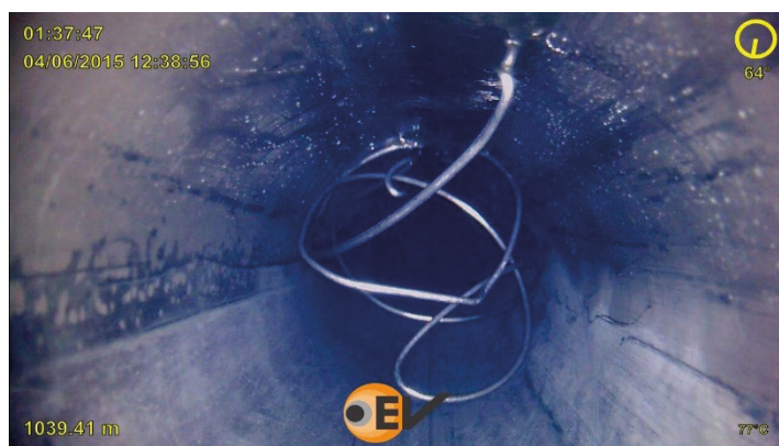
Figure 3: A short length of slickline cable located below the cutter after its successful retrieval
